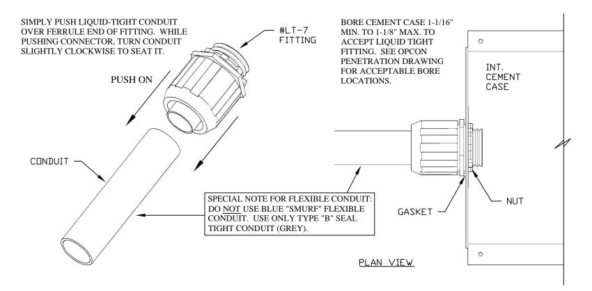
ARLINGTON #LT-7 LIQUID-TIGHT FITTING MUST BE USED FOR ELECTRICAL AND LOW VOLTAGE PENETRATIONS ON CEMENT CASE. OTHER FITTINGS HAVE NOT BEEN TESTED OR APPROVED; AND MAY CAUSE LEAKS THAT MAY VOID WARRANTY.
